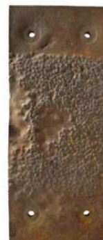
Used KenCast apron plate with minimal wear after 74,000 tons
